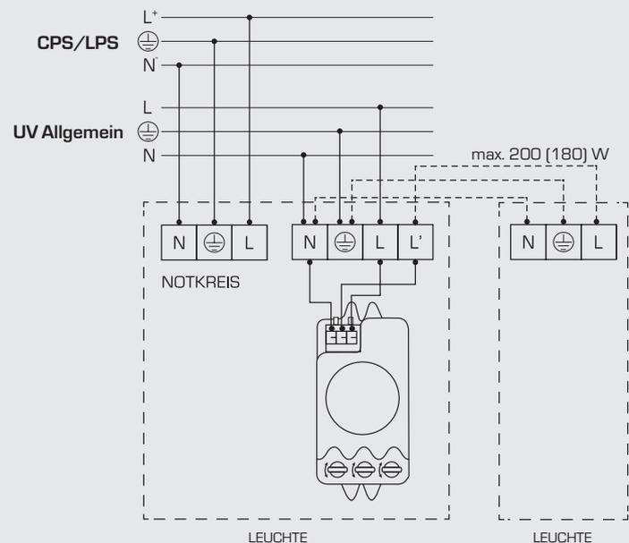
CPS / LPS ... Central Power Supply System (Zentralanlage) / Low Power Supply System (Gruppenanlage)
